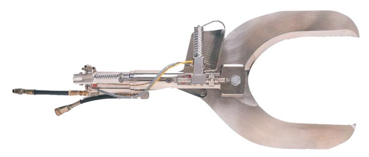
The Jarvis Model 50CL - hydraulically powered forequarter and loin dropper.
